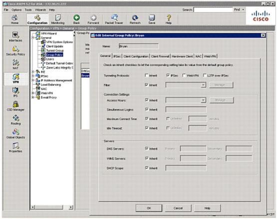
3. Once in the **General** tab, undo the **Inherit** check box for **Simultaneous Logins** under **Connection Settings**. Choose an appropriate value in the field.
