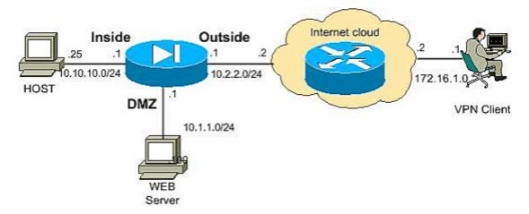
Check that the Split Tunnel, NO NAT configuration is added in the head-end device to access the resources in the DMZ network.
